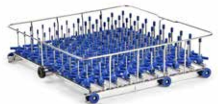
IXA: Injector rack, short injectors, 76 mm (3") tall, jets 2 mm diameter
